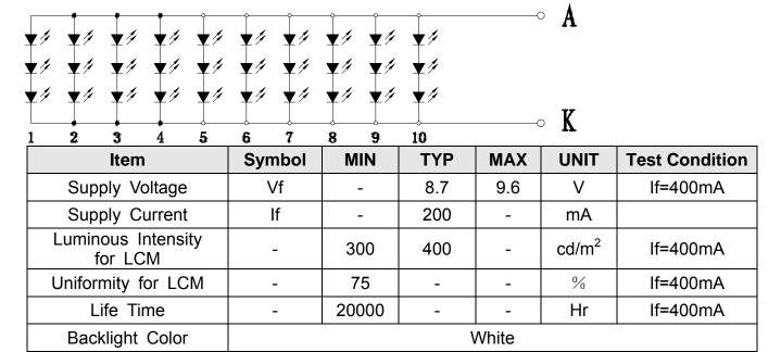
Note 1: The LED Supply Voltage is defined by the number of LED at Ta=25 $^{\circ}$ C and IL = 400mA.
