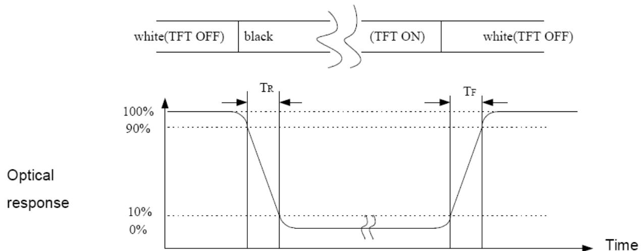
**Note (4) Definition of optical measurement setup**
